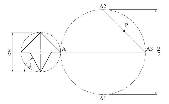
The given figure shows the design of a logo for a hat shop. Draw the given logo and then locate the points A, A1, A2, A3, P and the line A-A3 as shown.
