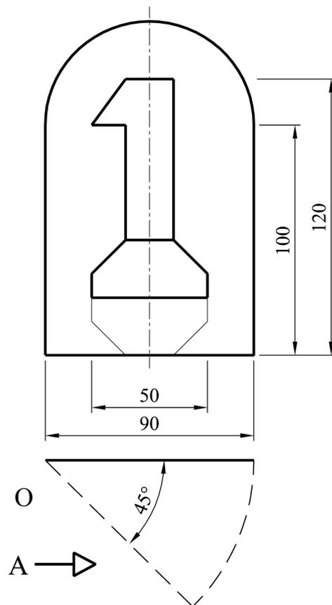
**3.** The axonometric axes required for the isometric projection of a bread bin are shown.
