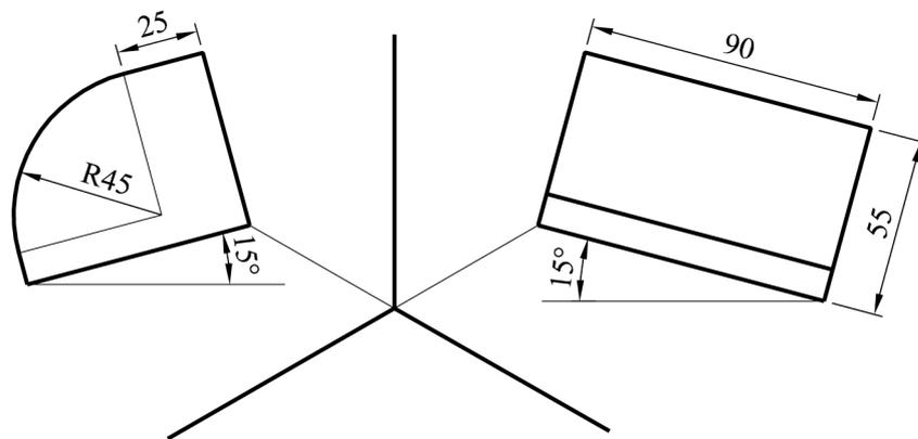
**4.** The elevation and end view of a design for an American style post box are shown.
