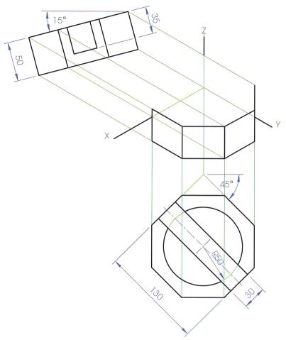
4. The figure below shows the incomplete isometric projection of a bird feeder using the axonometric axes method. The front and side elevations, which are identical, are also shown in their required positions.
