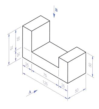
Build the object from 25 mm cubes as shown above. View the model from the viewing direction to help you visualise the solution.
