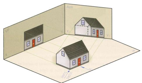
The line of intersection between the auxiliary vertical plane and the horizontal plane is called the  $X_1Y_1$  line and is the new ground line.
