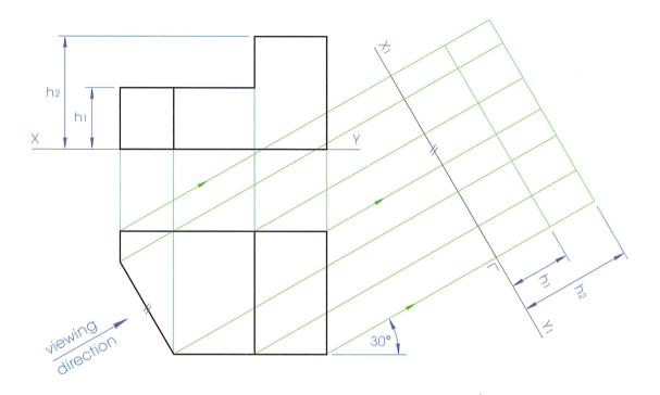
**6.** Line in the auxiliary elevation as shown below.
