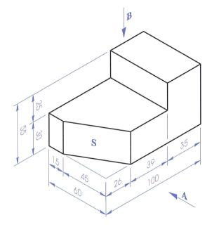
1. Consider the pictorial shown below. The true shape of surface S will appear in an auxiliary elevation in which the viewing direction is at right angles to the surface S, as indicated.
